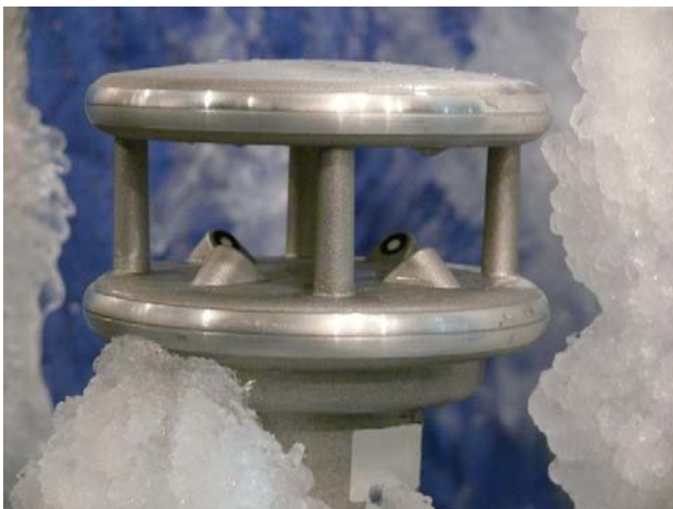
Ultrasonic anemometers with 200 W high power heating for cold climate applications. Economic compact versions without heating
