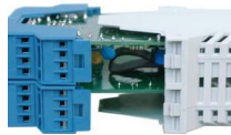
4a. At ZX4TE insert both units simultaneously. Both printed circuit boards are connected with a flat cable at the reverse side.
