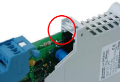
4. Disconnect 24VDC-supply and close the box. Attention! You have to control the fitting in the rails
