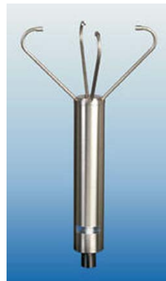
Ultrasonic anemometers for wind speed, wind direction and virtual temperature measurements. RS 232, RS 422, RS 485, NMEA or 4-20 mA output
